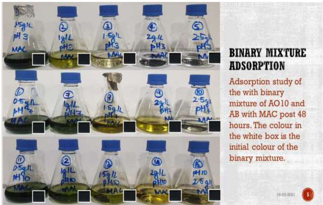
Figure 2. Simultaneous adsorption of two dyes (acid orange AO and acid blue AB) using untreated activated carbon (MAC)
