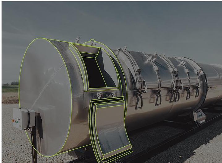
Invessel Composter with individual compartments ( In Fabrication)
